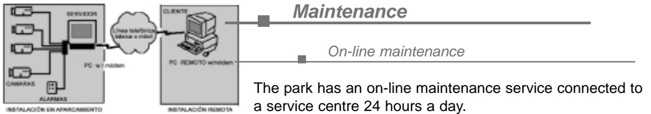
A high level language software monitorizes via modem the history of operations, control of images, checking of alarms, modification of data in the memory, the condition of the receptacles and also makes general verification tests of the status of the park. All this in **real time and remotely**.
